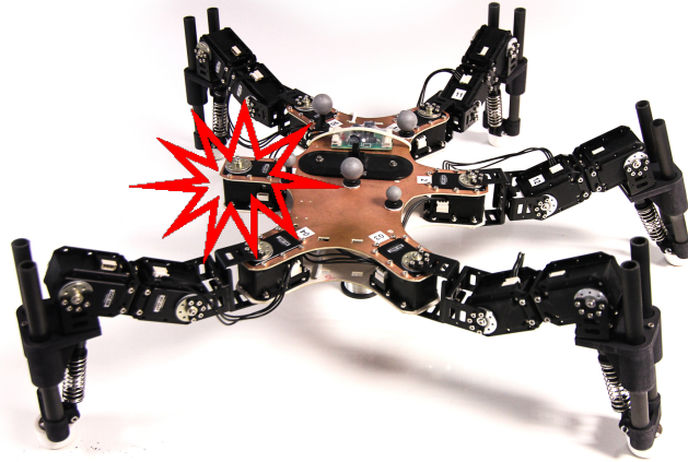
Figure 3.14: Physical damaged hexapod robot. The middle right leg is removed.
