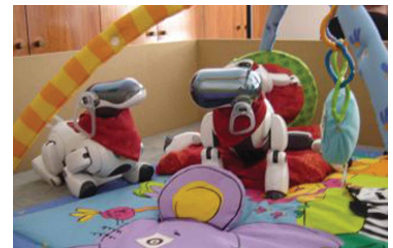
Figure 1.3: The Playground experiment (Oudeyer and Kaplan, 2006): a robot chooses its activities over time, according to its learning progress. Activity include grasping and touching objects, as well as communicating with a peer.
