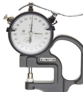
Figure 2.17: Thickness gauge
