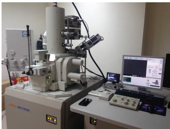
Figure 2.27: Scanning electron microscopy JEOL JSM - 7600F (Laboratory of Electron Microscopy and Microanalysis, HUST)
