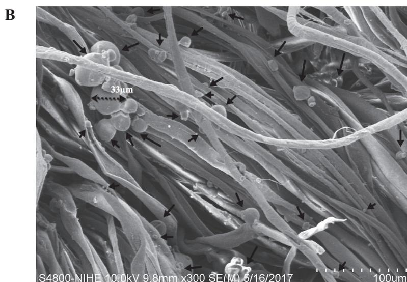
Figure 3.30: SEM images of the lower surface of the fabrics B1 (A) and B5 (B)
