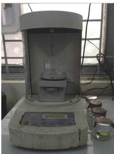
Figure 2.4: Tensiometer SEO-DST30M (Surface & Electro-Optics)
