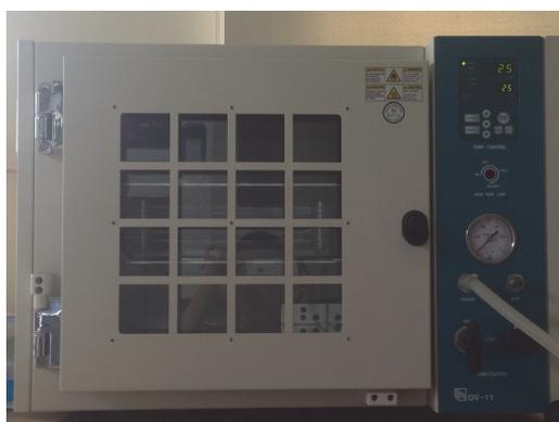
Figure 2.26: Vacuum drier OV-11
