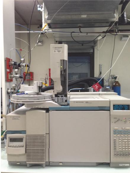
Figure 2.13: Gas chromatograph Agilent Technology 6890N
