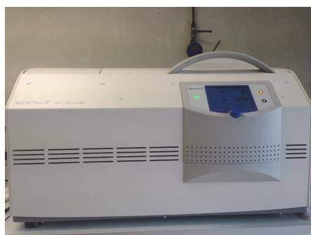
Figure 2.7: Centrifuge G-16KS of Sigma
