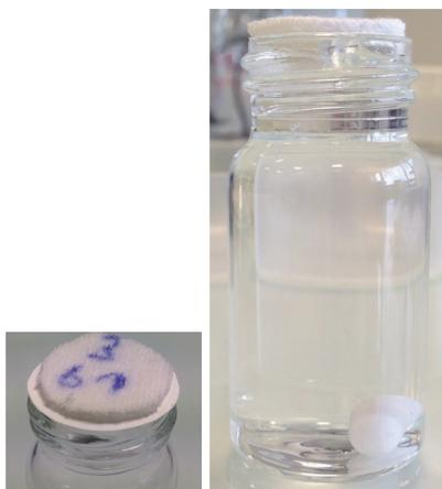
Figure 2.22: Glass jar simulating Franz diffusion cell
