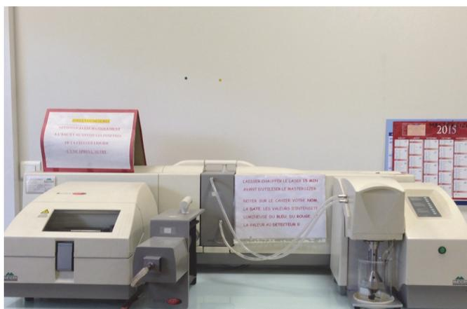
Figure 2.10: Mastersizer 2000, Malvern Instruments
