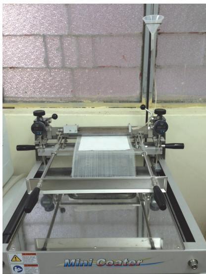
Figure 2.25: Coating equipment Mini Coater (DaeLim Starlet Co.,Ltd)
