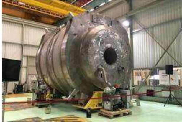
Figure 1: The MRI magnet of the NeuroSpin CEA research centre, Saclay, France, weights 130 tons and produces a magnetic field of 11.7 Tesla.
