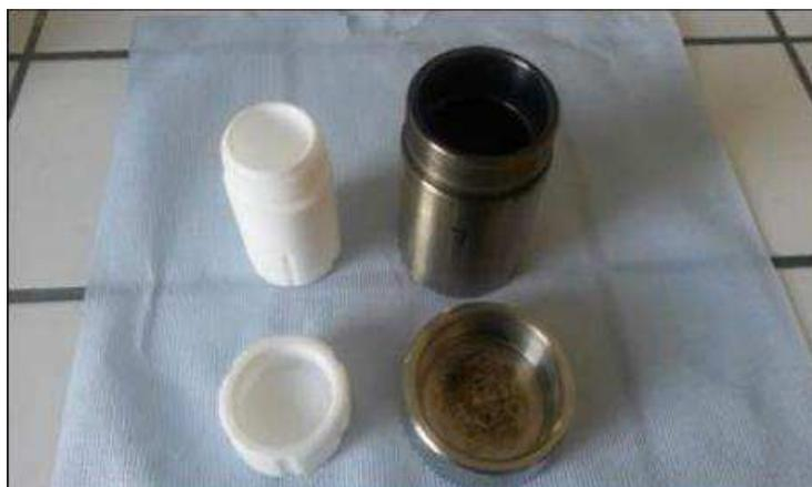
Figure 29: Stainless steel autoclave (right) and the Teflon container (left)
