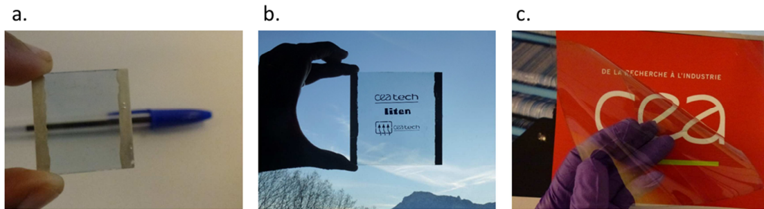
Figure III.2. Picture of PEDOT:Sulf deposited on (a) a 2.5 cm x 2.5 cm glass substrate with silver paints for contacts, (b) a 10 cm x 10 cm glass substrate and (c) a 10 cm x10 cm flexible PET substrate.
