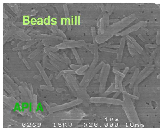
Figure 141: SEM of API A obtained with bead mill having d_{50} = 125 nm.
