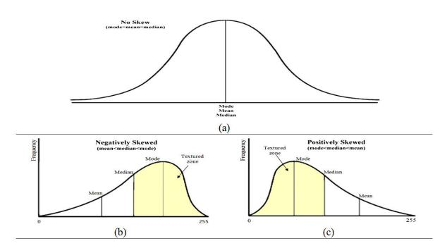
Figure 39: Diagram of (a) normal distribution, (b) negatively skewed distribution and (c) positively skewed distribution of gray-scale intensities.
