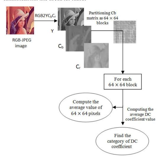
Figure 33: The structure of system initialization
