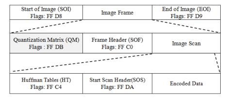
Figure 16: Syntax of JPEG file structure.
