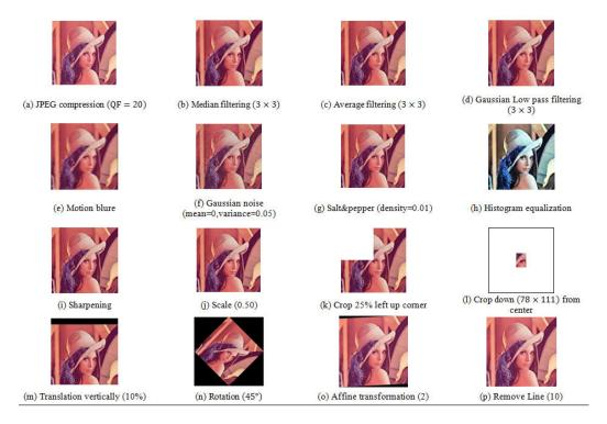
Figure 38: The consequences of applying different attacks on watermarked color Lena image.
