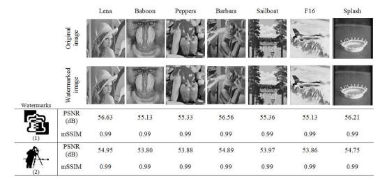
Figure 47: Imperceptibility results of blind image watermarking approach based on texture analysis using TOPSIS method on set of gray-scale images.
