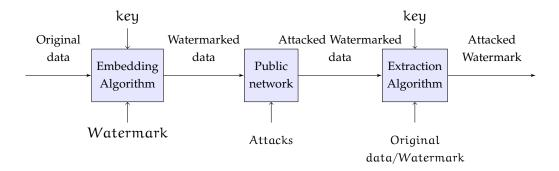
Figure 10: Main components of watermarking schemes.
