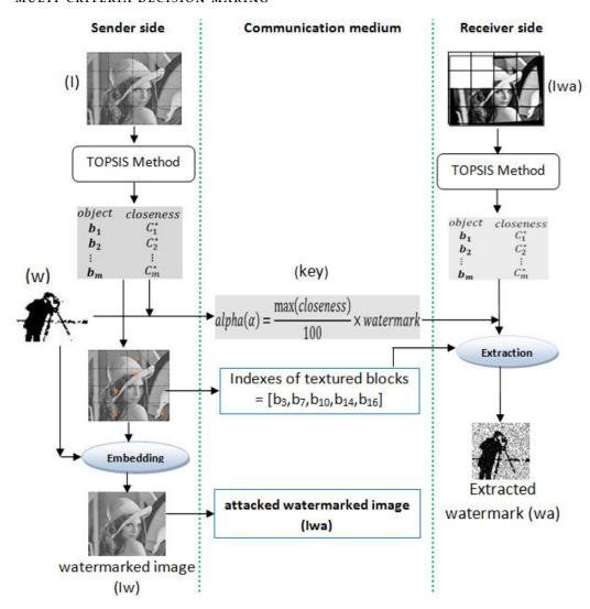
Figure 45: General framework of blind image watermarking approach based on texture analysis using TOPSIS method.
