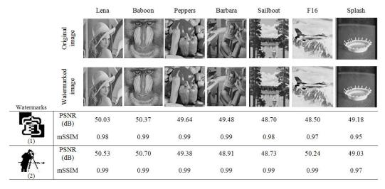
Figure 53: Imperceptibility results of semi-blind image watermarking approach based on texture analysis using FPM method on set of gray-scale images.
