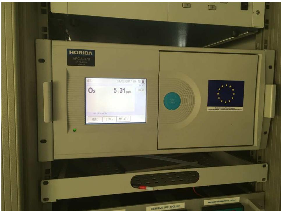
**Figure 2-12 Photo view of the APOA-370 O<sub>3</sub> monitor**
