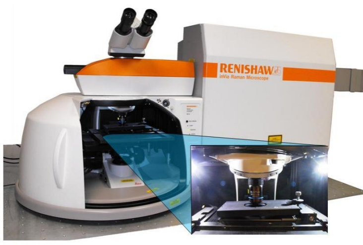
Fig. 2.7: The Renishaw inVia confocal Raman microspectrometer, the zoomed in photo is the sampling platform.
