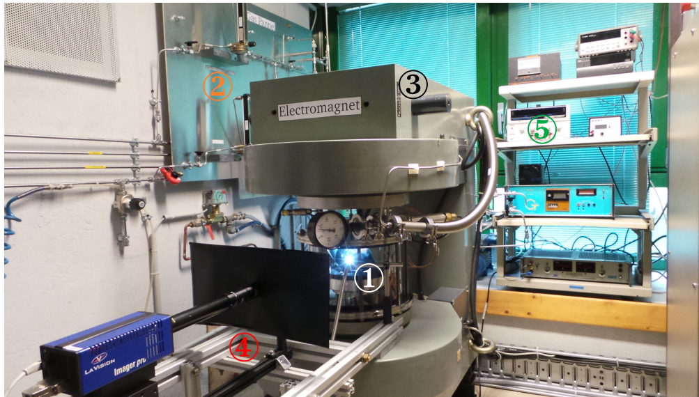
Figure III.D.2 – Photograph of the real experimental test-bench, with the 5 distinct working areas. Note that the electromagnet power supply and the computer workstation are not represented.
