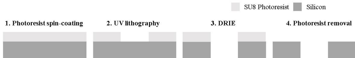
Figure III.12. Schematic representation of the fabrication process of the shadow mask.
