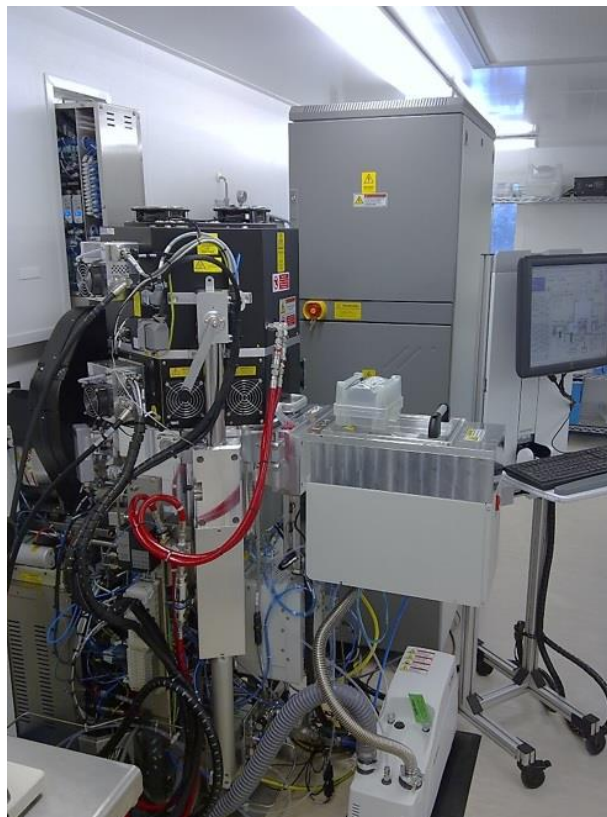
Figure III.9. Photo of ICP DRIE Rapier Omega LPX machine.
