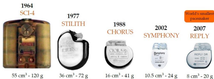
Figure I.8. Miniaturization of the pacemakers during the last 50 years [Deterre, 2013].
