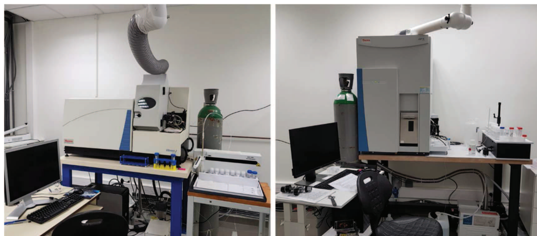
Figure 24: Two analytical equipments used in this study. Left: SQ ICP-MS and right: TQ ICP-MS.
