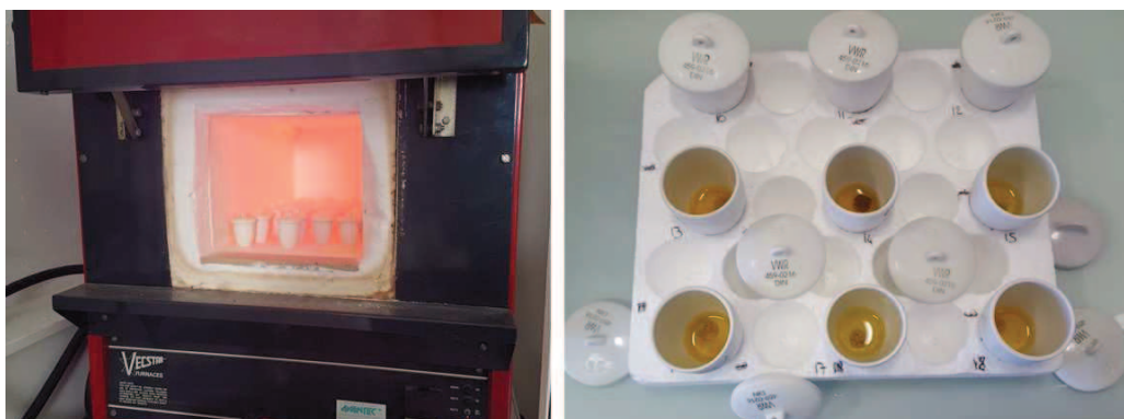
Figure 25: Ashing of the samples in the muffle furnace (left) and acid addition to cooled crucibles (right).
