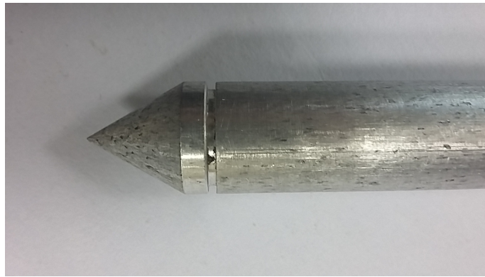
Figure 5.5: Photograph showing the pile surface after a typical test in the mini-calibration chamber
