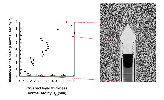
**Figure 6.14:** Evolution of the thickness of the layer of soil alongside the pile where grain crushing occurs and vertical slice showing this layer after pile installation during test P-GLAG-09
