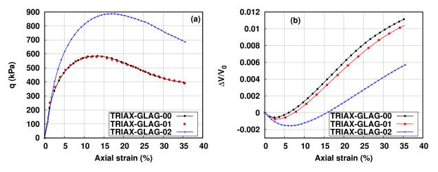
**Figure 4.5:** a) Deviatoric response of Glageon sand and b) Volumetric deformation curves for different confining pressures (100 kPa and 200 kPa)
