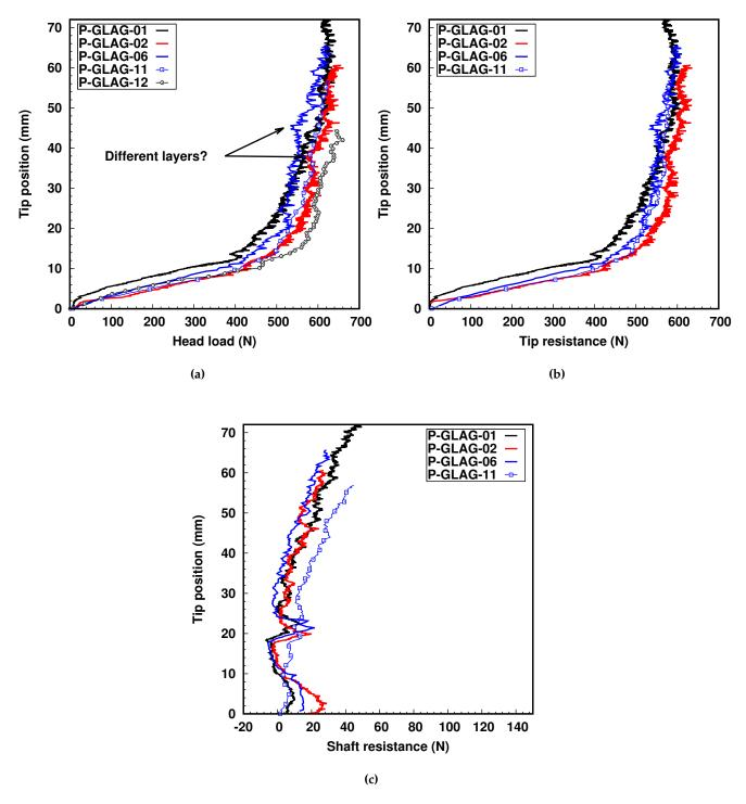
**Figure 5.4:** Load profiles during pile installation for different tests showing the reproducibility of the results (initial relative density between 85 % and 110 %): a) head load, b) tip resistance and c) shaft resistance. Note that the tip resistance and shaft resistance could not be recorded during test P-GLAG-12
