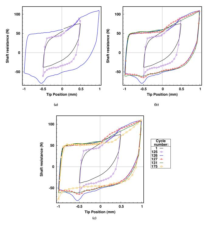
**Figure 5.15:** Evolution of shaft resistance when changing the amplitude of cycles from  $\pm 0.5mm$  to  $\pm 1.0mm$ : a) maximum peak shaft resistance "kept in memory" at  $\pm 0.5mm$ , b) smoothing of the first maximum peak shaft resistance and c) new maximum peak shaft resistance reached at  $\pm 1.0mm$  - test P-GLAG-14
