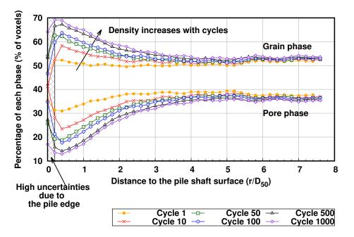
**Figure 6.20:** Radial evolution of grain (without fines) and pore phases volume during loading cycles for test P-GLAG-03 (amplitude of displacement  $\pm 0.5$  mm, initial relative density of 84 %). The x-axis scale is such that a radial distance of 7 is equal to one pile radius. For a given curve, each symbol represents one measurement obtained by thresholding the gray-scale image at a distance r from the shaft (over a cylindrical subdomain as defined in Section 3.3)
