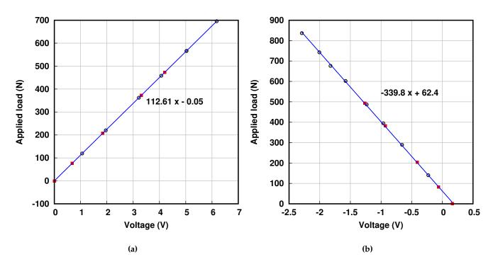
**Figure 4.9:** Calibration of the load measured by a) the head load sensor (total load applied to the pile) and b) the strain gauges (tip load). Full symbols represent compression and empty symbols represent tension
