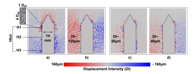
**Figure 6.15:** Typical individual grain displacements from discrete DIC, plotted in a vertical plane passing through the pile axis and showing the evolution of displacement intensity (DI) during loading cycles: a) vertical displacements, b) horizontal displacements between cycles 10 and 50; c) vertical displacements, d) horizontal displacements between cycles 500 and 1000. These results are from test P-GLAG-03 (amplitude  $\pm 0.5$  mm)
