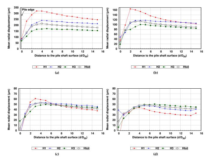
**Figure 6.17:** Mean radial displacements obtained from discrete DIC for different loading stages: a) cycles 1-10, b) cycles 10-50, c) cycles 50-100 and d) cycles 500-1000. Radial displacements are averaged within a toroidal subdomain of soil obtained by revolution of the rectangular cross-section shown in 6.15a. These results are from test P-GLAG-03 (amplitude  $\pm 0.5$  mm)
