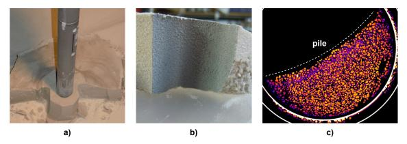
**Figure 2.9:** a) Moulding of the sand before extraction, b) frozen sample, and c) slice showing fine particles at the interface obtained by x-ray tomography, after(Silva et al., 2013)
