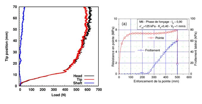
**Figure 5.1:** Evolution of the loads applied on the pile during the initial embedment for test P-GLAG-01
