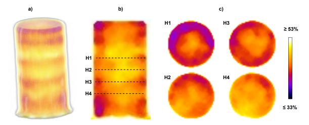
**Figure 4.15:** Porosity at the initial state for test P-GLAG-16: a) 3D field of porosity, b) Vertical slice through the 3D field, and c) horizontal slices taken at different elevations through the 3D field (H1, H2, H3, H4)
