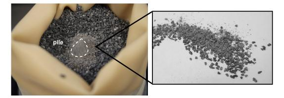
**Figure 6.13:** Photograph of the sample when the setup was disassembled after pile installation. A light-gray powder can be seen around the pile, which is delimited by the dashed line. A zoom into the material sampling at the interface shows the powder produced by grain crushing
