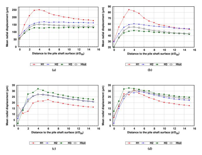
**Figure 6.18:** Mean radial displacements obtained from discrete DIC for different loading stages: a) cycles 1-5, b) cycles 10-20, c) cycles 70-100 and d) cycles 100-150. Radial displacements are averaged within a toroidal subdomain of soil obtained by revolution of the rectangular cross-section shown in 6.15a. These results are from test P-GLAG-09 (amplitude  $\pm 1.0$  mm)
