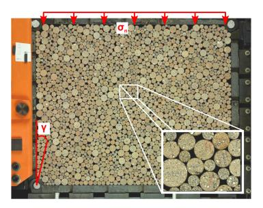
**Figure 5.19:** Image of an isotropically compressed sample in the  $1\gamma 2\epsilon$  device, with zoom on a small amount of grains to show the speckle pattern on their visible face, after Tolomeo et al. (2017) (the frame is 599.4 mm x 444.7 mm).  $\sigma_n$  and  $\gamma$  are the vertical stress and the shear angle imposed, respectively
