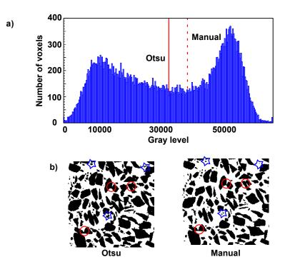
**Figure 3.8:** Selection of a manual threshold to identify (and next separate) grains in the framework of discrete DIC. a) Histogram showing the manual threshold and the Otsu threshold. b) Differences between the binary data produced with Otsu and manual threshold values: red circles show the difference in the size of the contacts between grains and the blue stars show that with a manual threshold the grain phase is intentionally underestimated
