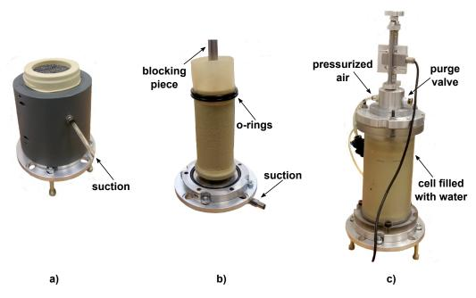
**Figure 4.13:** Different steps of sample preparation: a) sand deposition within a cylindrical mold, b) mold removal for the measurement of sample height and diameter and c) cell assembly
