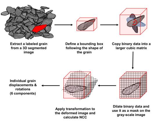
Figure 3.14: Flow chart showing the main steps of the implementation of the 3D discrete DIC in Tomowarp2
