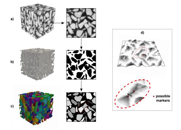
**Figure 3.10:** Diagram showing the segmentation process on a sub-volume. a) Gray-scale sub-volume and a 2D slice taken from it. b) Sub-volume and slice after binarization. c) Sub-volume and slice segmented and labeled showing a grain split into two particles (over-segmentation). d) 2D Euclidean distance map of the binarized slice displayed as a landscape and zoom showing two possible local maxima detected as markers for watershed segmentation
