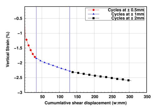
**Figure 5.18:** Evolution of the axial shear strain with cumulative shear displacement when changing the amplitude of cycles from  $\pm 0.5mm$  to  $\pm 1.0mm$  and to  $\pm 2.0mm$  (associated with the test presented in Figure 5.17)
