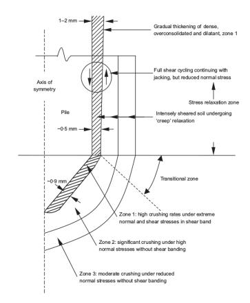
**Figure 2.8:** Schematic development of concentric zones around the pile shaft involving different degrees of particle crushing and their relationship to stress regime (not to scale), from Yang et al. (2010)
