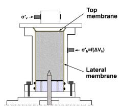
**Figure 7.1:** Sketch showing a possible modification of the mini-calibration chamber for the application of active radial boundary conditions
