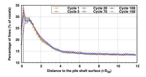
**Figure 6.25:** Radial evolution of the quantity of fines during loading cycles for test P-GLAG-09 (amplitude of displacement  $\pm 1.0$  mm, initial relative density of 85 %). The x-axis scale is such that a radial distance of 7 is equal to one pile radius. For a given curve, each symbol represents one measurement obtained by thresholding the gray-scale image at a distance r from the shaft (over a cylindrical subdomain as defined in Section 3.3
