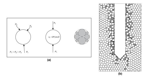
**Figure 2.11:** a) Maximum coordination number for a particle to be able to break; loading conditions on a particle assumed to be equivalent to the one of a diametrical compression test; configuration after breakage and b) Evolution of average radial stresses in representative cycles: strain (-0.1, +0.1%), from Lobo-Guerrero and Vallejo (2005)
