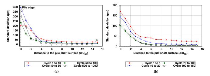
**Figure 6.19:** Evolution of the standard deviation of the radial displacements for the elevation H1 during cycles: a) test P-GLAG-03 of Fig. 6.17, b) test P-GLAG-09 of Fig. 6.18
