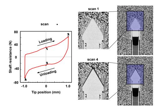
**Figure 6.27:** Sketch showing the high densification of the sand ahead of the pile tip during test P-GLAG-11. The numbers placed on the curve showing the typical evolution of shaft resistance indicate when the loading was interrupted for x-ray scanning. The two vertical slices (on the right) were taken through the 3D images recorded after the tenth cycle, when the tip was at 0 mm (scan 1) and at -1.0 mm (scan 4). The zooms into the slices illustrate the densification at the tip
