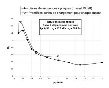
**Figure 5.14:** Evolution of the degradation of shaft resistance with the amplitude of loading cycles, from Le Kouby (2003). The degradation factor  $D_{\tau}$  was defined as the ratio between the limit shaft resistance after and prior to cyclic loading
