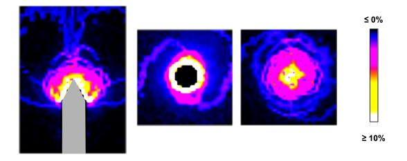
**Figure 3.15:** Example of slices through the maximum shear strain field obtained with a tri-linear spline interpolation in the sub-pixel search. Please note that the color contrast was enhanced for clarity
