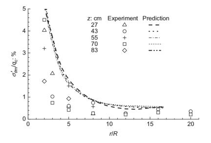
**Figure 2.10:** Comparison of numerical circumferential stresses at h/R = 0.5 level above the tip during penetration and experimental results obtained by Jardine et al. (2013), from Zhang et al. (2014)
