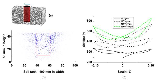
**Figure 2.13:** a) Configuration of soil tank and pile; b) Incremental soil displacements at the end of the given cycle (mm): strain (-0.1, +0.1%), 1st-50th cycles; c) Evolution of average radial stresses in representative cycles: strain (-0.1, +0.1%), after Cui and Bhattacharya (2016)
