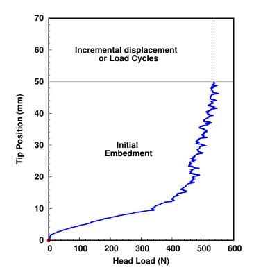
Figure 4.16: Typical head load profile during pile installation
