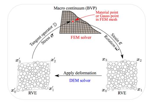
**Figure 2.14:** Schematic illustration of the hierarchical computational framework for multi-scale modeling of granular material, from Zhao (2008)
