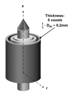
**Figure 3.12:** Local density changes at the interface: sketch showing the subdomains over which the percentage of each phase (grains, fines and pores) is estimated. These subdomains are hollow cylinders with a thickness of 5 voxels (*i.e.*, 0.2 mm), coaxial to the pile
