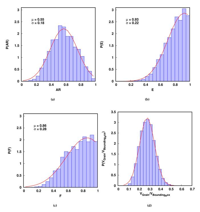
**Figure 4.3:** Preliminary shape analysis of Glageon sand grains based on the bounding boxes: a) aspect ratio, b) elongation and c) flatness. d) Ratio between the volume of the grains over the volume of their bounding box. The red curve show the Gaussian fit associated with a deviation  $\sigma$  and a mean  $\mu$
