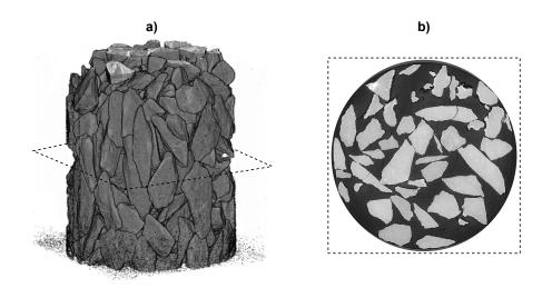
**Figure 4.1:** a) 3D-reconstructed volume of an œdometer sample of Glageon sand (granular fraction: 1.250 - 1.600 mm) at ESRF, Grenoble, by Dano and coworkers (2018) at a voxel size of 6.5  $\mu$ m. b) Horizontal slice taken through the reconstructed volume showing the angularity of Glageon sand grains
