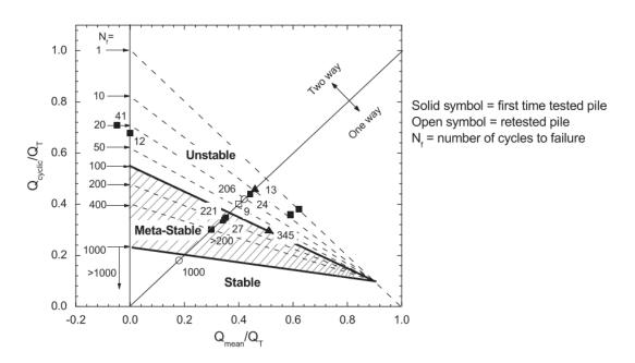
**Figure 2.3:** Interaction diagram for full-scale piles, from Jardine and Standing (2000). Numbers within the graph area represent the number of cycles for each test
