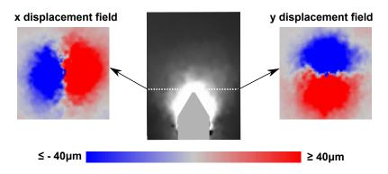
**Figure 6.2:** Horizontal slices taken within the 3D field of horizontal displacements in both x and y directions. These results were obtained with continuum DIC, for the increment 2-3 mm of test P-GLAG-00
