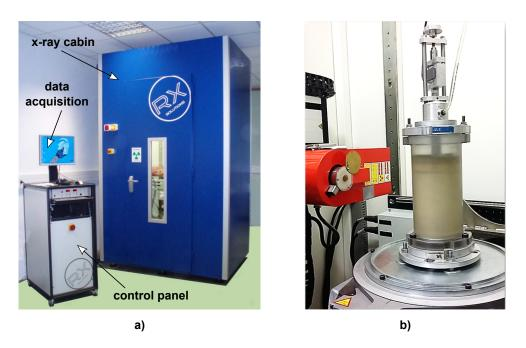
**Figure 3.1:** a) 3SR x-ray device including the cabin and the control panel. b) Setup installed in front of the x-ray source within the cabin
