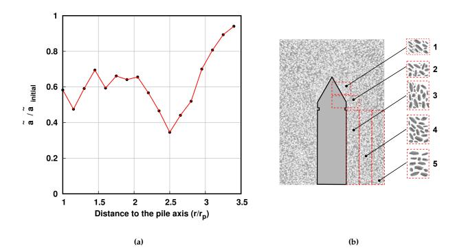
**Figure 6.9:** a) Radial evolution of the ratio between  $\tilde{a}$  and  $\tilde{a}_{initial}$  showing the change in anisotropy prior to and after pile installation. b) Schematic illustrating the fabric formed following pile penetration at different locations around the pile tip and the pile shaft. In this figure,  $\tilde{a}_{initial}$  was obtained over all grains at the initial state and its value is 0.095
