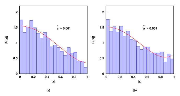
**Figure 6.10:** Distribution of grains orientations and its representation using Legendre polynomials expansion truncated at the 4th order after pile installation. The level of anisotropy was estimated by determining  $\tilde{a}$  over two subdomains located around the pile tip corresponding to the regions 1 and 2 in Figure 6.9b
