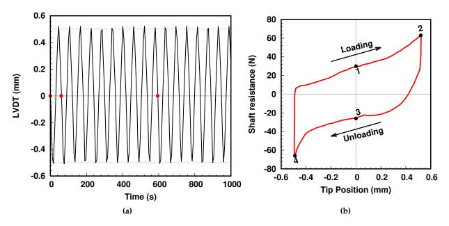
**Figure 4.17:** a) Typical displacement imposed to the pile during loading cycles; b) Typical shaft resistance evolution within a cycle. (red and black dots represent an x-ray scan acquisition)
