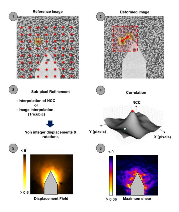
**Figure 3.13:** Flow chart explaining the different steps of continuum DIC implemented in Tomowarp2 (existing code employed in this work). The example is given in 2D for clarity and show the displacement field and the maximum shear strain field for an incremental displacement of the pile tip of 1.0 mm
