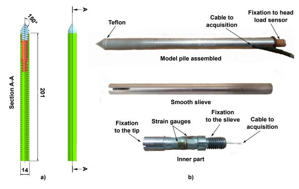
**Figure 4.8:** Design of the model pile: a) drawing made by DOERLER Mesures and b) schematic of the different parts of the model pile
