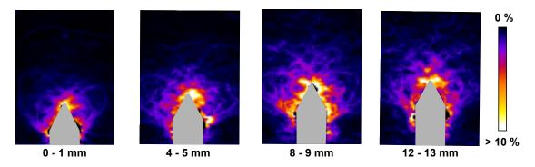
**Figure 6.12:** Vertical slices through the 3D deviatoric strain field (*i.e.*, maximum shear strain) calculated from continuum DIC kinematics for test P-GLAG-00
