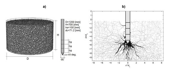
**Figure 2.12:** a) View of the virtual calibration chamber and the model pile. b) Contact normal forces exceeding average normal force (the lines thickness is proportional to the magnitude of the normal force), from Butlanska et al. (2014)
