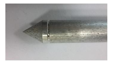
**Figure 5.5:** Photograph showing the pile surface after a typical test in the minicalibration chamber
