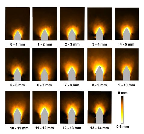
**Figure 6.4:** Vertical slices taken through the 3D field of vertical displacements obtained with continuum DIC (node spacing: 20 pixels, correlation window size: 40 voxels) for an incremental displacement of the pile tip of 1 mm until a maximum displacement of 14 mm (test P-GLAG-00)
