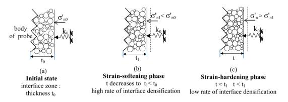
**Figure 2.7:** Schematic explaining the different phases in shaft friction evolution in the case of low consolidation stress, from Bekki et al. (2013)
