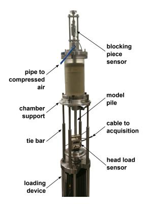
Figure 4.14: Experimental arrangement before pile installation for a test conducted outside the tomograph
