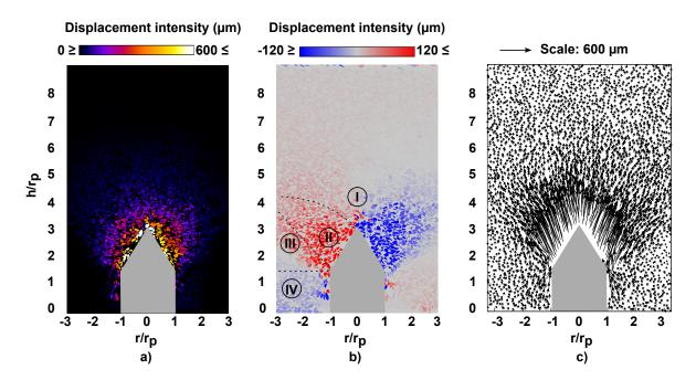
**Figure 6.6:** Typical individual grain displacements from discrete DIC, plotted in a vertical plane passing through the pile axis, when the pile tip moved up from h = 37mm to h = 38mm (increment 2-3 mm): a) vertical displacements; b) horizontal displacements; c) individual displacement vectors for the same loading increment. These results are from test P-GLAG-00. Dashed lines delimit the different zones of displacement
