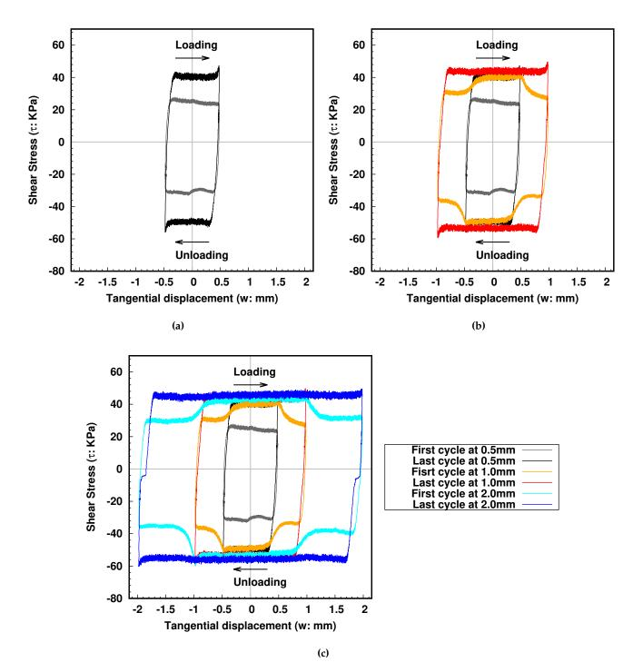
**Figure 5.17:** Evolution of the shear stress when changing the amplitude of cycles from  $\pm 0.5mm$  to  $\pm 1.0mm$  and to  $\pm 2.0mm$ : a) maximum peak shear stress visible at  $\pm 0.5mm$ , b) smoothing of the first maximum peak shear stress and new maximum peak shear stress visible at  $\pm 1.0mm$ , c) smoothing of the second maximum peak shear stress and new maximum peak shear stress visible at  $\pm 2.0mm$ . Please, note that the key is common to the three plots
