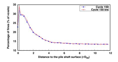
**Figure 6.26:** Radial evolution of the quantity of fines for two different x-ray scans recorded after 150 cycles during test P-GLAG-09. The measurements on two scans show the reproducibility of the methodology described in Section 3.3
