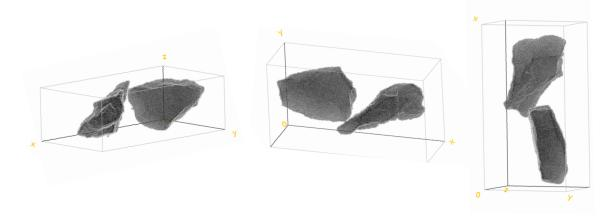
**Figure 4.4:** Example of two grains extracted from the reconstructed volume of Figure 4.1. The grains are displayed in different orientations to show that one is rather elongated and the other one platy but both have a longer dimension
