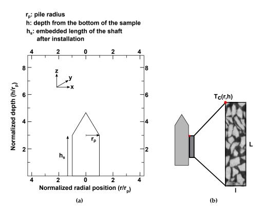
**Figure 6.3:** a) Coordinate reference system for image analysis data reporting. b) Schematic showing how a subdomain is defined for averaging micro-scale measurements on the circumference of the sample
