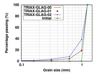
**Figure 4.6:** Grain size distribution before and after triaxial compression at different isotropic confining pressure on dense sample of Glageon sand
