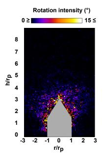
**Figure 6.7:** Individual grain rotations plotted in a vertical plane passing through the pile axis, when the pile tip moved up from h = 37mm to h = 38mm (increment 2-3 mm) during test P-GLAG-00. The color scale represents the rotation intensity in degrees
