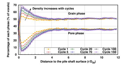
**Figure 6.21:** Radial evolution of grain (without fines) and pore phases volume during loading cycles for test P-GLAG-09 (amplitude of displacement  $\pm 1.0$  mm, initial relative density of 85 %). The x-axis scale is such that a radial distance of 7 is equal to one pile radius. For a given curve, each symbol represents one measurement obtained by thresholding the gray-scale image at a distance r from the shaft (over a cylindrical subdomain as defined in Section 3.3)
