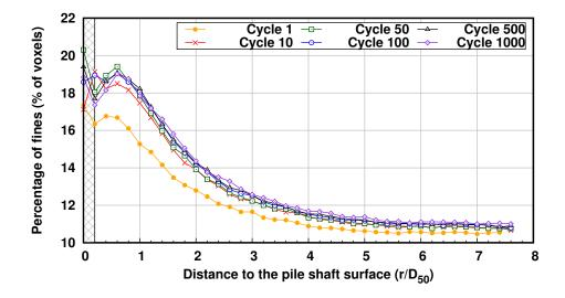
**Figure 6.24:** Radial evolution of the quantity of fines during loading cycles for test P-GLAG-03 (amplitude of displacement  $\pm 0.5$  mm, initial relative density of 84 %). The x-axis scale is such that a radial distance of 7 is equal to one pile radius. For a given curve, each symbol represents one measurement obtained by thresholding the gray-scale image at a distance r from the shaft (over a cylindrical subdomain as defined in Section 3.3
