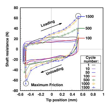
Figure 5.9: Evolution of shaft resistance during displacement-controlled loading cycles for test P-GLAG-02 (amplitude of  $\pm 0.5$  mm)
