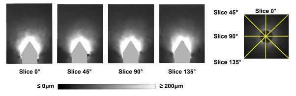
**Figure 6.1:** Vertical slices taken at different angular position within the 3D field of vertical displacements. These results were obtained with continuum DIC, for the increment 2-3 mm of test P-GLAG-00
