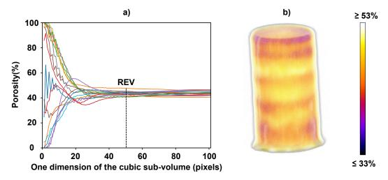
**Figure 3.11:** Example of sample characterization at the initial state. a) Evolution of the porosity measurement as the cubic sub-volume on which it is measured increases from one voxel to a cube measuring  $100 \ pixel^3$  and selection of the REV size. b) 3D porosity field for the selected REV of  $50 \ pixel^3$
