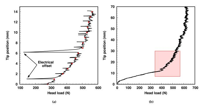
**Figure 5.7:** a) Incremental loading steps applied to the pile during scanning for test P-GLAG-00. The circles represents the steps when the loading was interrupted for scanning. b) Sketch of the region of interest analyzed by x-ray tomography during pile embedment
