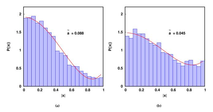
**Figure 6.8:** Distribution of grains orientations and its representation using Legendre polynomials expansion truncated at the 4th order (P(|x|) = 2p(x)) a) prior to and b) after pile installation
