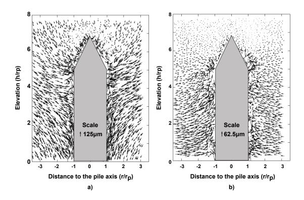
**Figure 6.16:** Individual displacement vectors obtained for the same loading increments as Figure 6.15, plotted in a vertical plane passing through the pile axis: a) between cycles 10 and 50 and b) between cycles 500 and 1000. Note that the scale is different in figures a and b
