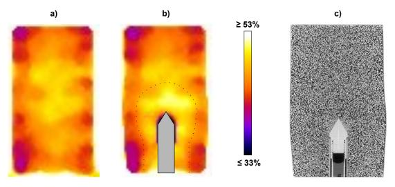
**Figure 6.11:** Vertical slices selected through the measured 3D field of porosity a) before and b) after pile installation, for test P-GLAG-16. c) Same vertical slice through the 3D reconstructed volume showing the global volume change of the sample after pile installation
