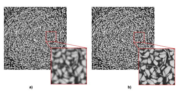
**Figure 3.4:** Horizontal slice taken through a 3D reconstructed image recorded in local tomography: a) before the correction of the misalignments and b) after correction in X-Act
