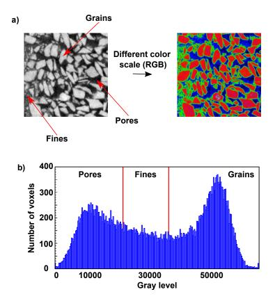
**Figure 3.6:** Illustration of the definition of the different phases in a gray image: a) Image subset (2D, 16 bit) recorded in local tomography showing grains, pores and fines. The same subset displayed with a different color scale helps differentiating the three phases (grains: red, pores: blue, fines: green). b) Histogram associated with the image subset indicating the two threshold values selected manually to isolate each phase
