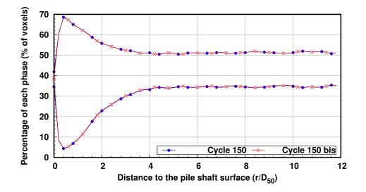
**Figure 6.23:** Radial evolution of grain (without fines) and pore phases volume for two different x-ray scans recorded after 150 cycles during test P-GLAG-09. The measurements done on two scans show the reproducibility of the methodology described in Section 3.3
