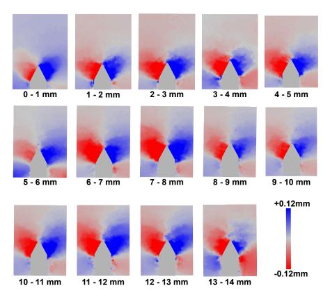
**Figure 6.5:** Vertical slices taken through the 3D field of horizontal displacements obtained with continuum DIC (node spacing: 20 pixels, correlation window size: 40 voxels) for an incremental displacement of the pile tip of 1 mm until a maximum displacement of 14 mm (test P-GLAG-00)
