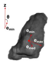
**Figure 3.16:** Scheme illustrating the measurement of the orientation  $\theta$  of a single Glageon grain.  $\vec{e_{min}}, \vec{e_{med}}$  and  $\vec{e_{max}}$  are the minimum, the intermediate, and the maximum eigenvectors of the inertia tensor, respectively
