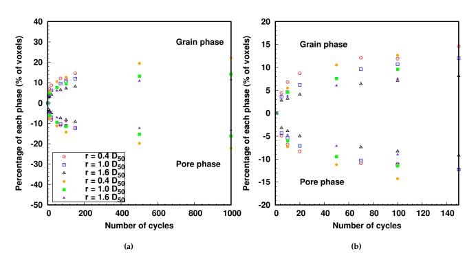
**Figure 6.22:** a) Density evolution at different distances "r" from the pile surface when increasing the number of loading cycles and b) zoom into the first 150 cycles. The results obtained for test P-GLAG-03 are plotted with filled symbols and the one obtained for test P-GLAG-09 are plotted with empty symbols. To meaningfully compare the two tests, the initial percentage measured for the first cycle was subtracted from all values
