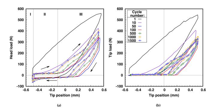
**Figure 5.8:** Evolution of a) head and b) tip load during displacement-controlled loading cycles for test P-GLAG-02 (amplitude of  $\pm 0.5$  mm). Arrows indicate the loading path within a single cycle
