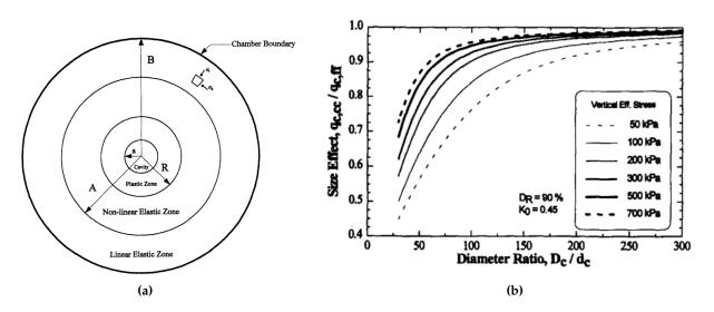
**Figure 5.6:** a) Different zones developing around the pile during cavity expansion and b) size effect curves for several vertical stress values (cc: calibration chamber, ff: free-field), after Salgado et al. (1998)
