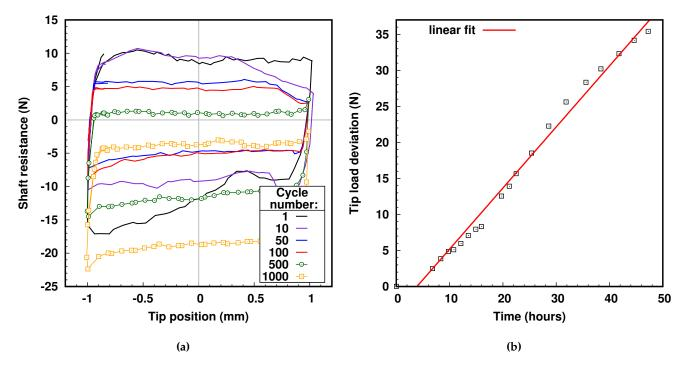
**Figure 5.11:** Deviation of the measurements given by the instrumented model pile: a) inconsistent shaft resistance values during test P-GLAG-05, b) tip load deviation during test P-GLAG-06 and its linear fit (inside the tomograph)
