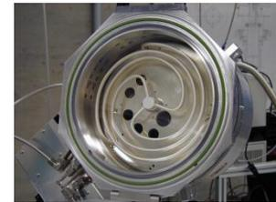
Source ICP antenne triple
