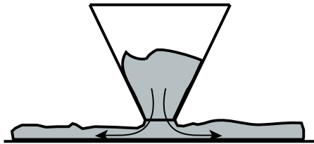
(a) Sketch illustrating the high flowability of modern concrete.
