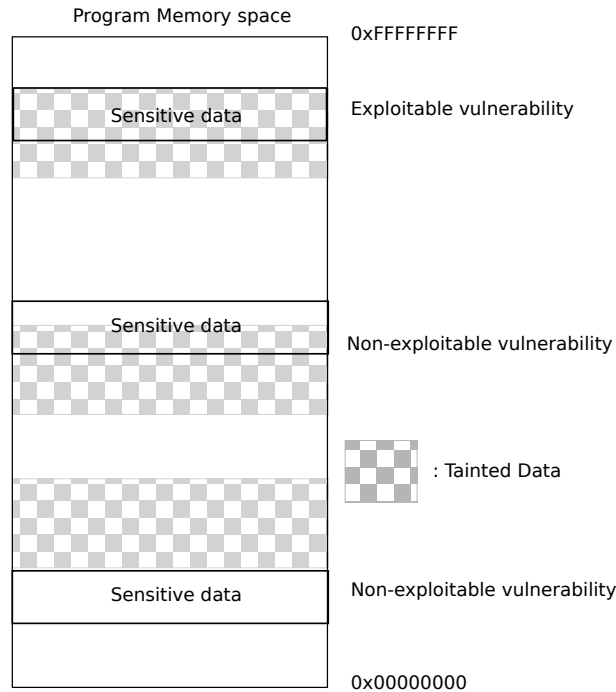
FIGURE 5.3: Exploitable vulnerability pattern. Sensitive memory erased with tainted data.
