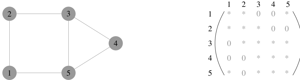
Figure 2.2 – Link between an undirected graph and the zeros in the matrix that encodes the considered dependencies.
