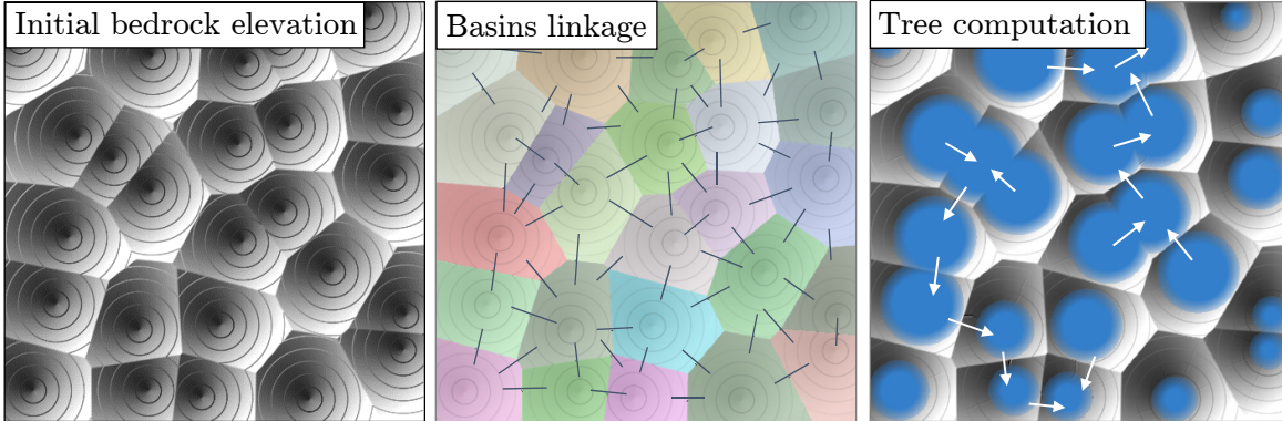
Figure 3.5: Illustration of the water flow resolution on a synthetic case. The initial terrain is computed thanks to a Voronoi diagram: a set of points at random locations are set to altitude 0, and the elevation is obtained by locally computing the distance to the nearest sample point (left). The basins are first segmented and each pair of basins are connected through a single pass (middle). Then, the minimum spanning tree algorithm is used to select some of these connections, giving the final flow direction. In the rightmost figure, the basins undergo a moderate erosion and we show the water level in blue.
