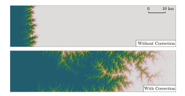
**Figure 3.11**: Simulation of erosion of 500 m high escarpment on a  $1024 \times 256$  terrain. The nodes of the leftmost column are the only 0 altitude boundary nodes. We show the result of 70 time steps of 1,000 years each, without (top) and with (bottom) connecting the lakes.
