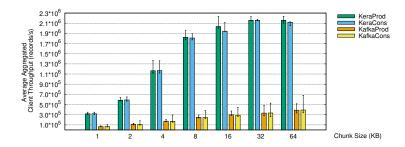
**Figure 8.7** – Evaluating the ingestion component when increasing the chunk/request size. Parameters: 4 brokers; 16 producers running concurrently with 16 consumers; number of partitions/streamlets is 16, 1 active group per streamlet; *request.size* equals *chunk.size* multiplied by 4 (number of partitions/streamlets per broker). On X we represent producer *chunk.size* (KB), for consumers we configure a value 16x higher.
