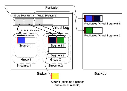
**Figure 7.3** – The virtual log technique for adaptive and fine-grained replication. In this example a stream with 2 streamlets is created and managed by one broker, with one backup used to replicate the stream. We create and maintain in-memory a log-based data structure to represent our virtual log that aggregates chunks of different groups of streamlets of a single stream. Optionally, the stream can be configured with more virtual logs that can be associated to its streamlets.
