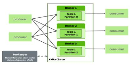
**Figure 5.2** – Static partitioning in Kafka (taken from [49]). Fixed partitioning can be a source of imbalance. Each partition is exclusively processed by one consumer.
