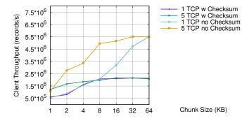
**Figure 8.6** – Impact of source record checksum computation on consumer throughput (one producer with one consumer running in parallel).
