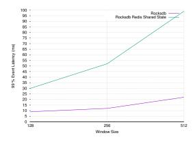
**Figure 4.5** – Event processing latency (99% percentile) for fixed event rate when varying the window size (off-heap versus shared). Rate of new events is 36. Heap size is 1 GB. Parallelism is one: all events correspond to the same window. Heap event latency is 5 milliseconds.
