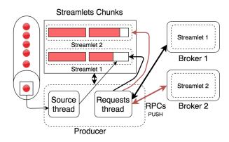
**Figure 8.1** – Producer architecture. The Source thread appends records to in-memory chunk buffers. The Requests thread batches one chunk for each streamlet (if the chunk is filled or a configurable timeout per chunk passed) in requests and pushes them to brokers.
