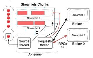
**Figure 8.2** – Consumer architecture. The Requests thread builds one request for each broker and pulls one chunk for each streamlet associated to the consumer. The Source thread consumes in-order one chunk per streamlet: it iterates the chunk and creates records. The source could push these records to other streaming operators for further processing.
