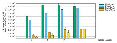
**Figure 8.10** – Horizontal scalability: increasing the number of nodes (brokers). Parameters: 32 producers running concurrently with 32 consumers; 256 partitions, 32 streamlets with 8 active groups per streamlet; *chunk.size* = 16KB; *request.size* = *chunk.size* multiplied by the number of partitions/active groups per node.
