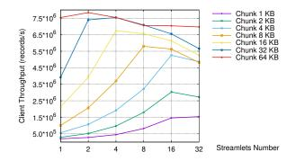
**Figure 8.3** – Single producer throughput (measured in million records per second) when increasing the chunk size and respectively the number of streamlets. The request size equals the chunk size multiplied by the number of streamlets. The pipelined producer (5 TCP requests) does not compute the record checksum.
