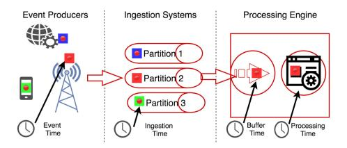
**Figure 7.4** – Current streaming architecture with pull-based consumers: records are collected at *event time* and made available to consumers earliest at *ingestion time*, after the events are acknowledged by producers; processing consumers continuously pull these records and buffer them at *buffer time*, and then deliver them to the processing operators, so results are available at *processing time*.
