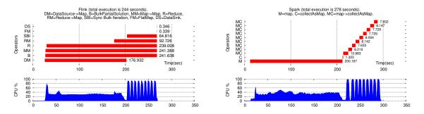
Figure 3.17 – K-Means operators and resource usage of Flink and Spark for 24 nodes, 10 iterations and 1.2 billion samples dataset. Resource usage elements not shown for similarity reasons: memory and disk utilization are less than 10%, total disk I/O (r+w) is less than 20 MB/s, and total network (r+w) is less than 30 MB/s.
