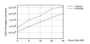
**Figure 8.13** – Increasing the number of active groups brings increased throughput (replication factor 1). 16 clients compete on streamlets configured with 1 and 4 active groups, while 4 virtual logs are used for replication.
