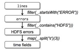
**Figure 3.2** – Lineage graph for a Spark query (taken from [120]). "Boxes represent RDDs and arrows represent transformations" [120].
