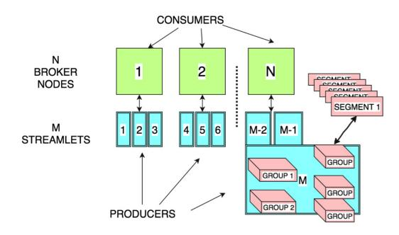
**Figure 6.2** – Semantic partitioning of streams with streamlets. A stream (also called distributed topic) is logically composed of a set of streamlets. At its turn, each streamlet is composed of an unbounded set of fixed-size sub-partitions called groups of segments.
