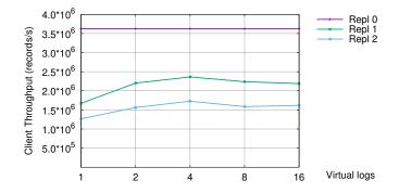
**Figure 8.16** – Increasing the number of virtual logs (16 clients, 8 streamlets, 4 brokers). 16 virtual logs correspond to the total number of active groups on a broker (2 streamlets per broker multiplied by 8 active groups)
