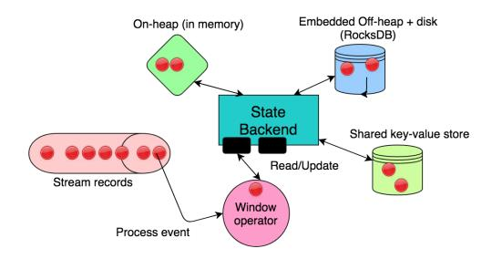
Figure 4.1 – State backend options for window-based streaming operations.
