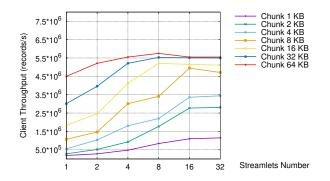
**Figure 8.5** – Single consumer throughput (measured in million records per second) when increasing the chunk size and respectively the number of streamlets. The request size equals the chunk size multiplied by the number of streamlets. The pipelined producer (5 TCP requests) does not compute the record checksum.
