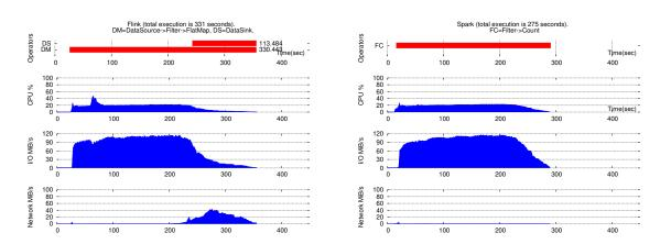
**Figure 3.12 –** Grep operators and resource usage. Flink (left) versus Spark (right), 32 nodes and 768 GB dataset. Similar memory usage, growing linearly up to 30%.
