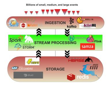
**Figure 2.1** – The usual streaming architecture is composed of three layers: data streams are first acquired by the *ingestion layer* and then they flow through the *processing layer* which relies on the *storage layer* for storing aggregated data, intermediate results or for archiving streams for later processing.
