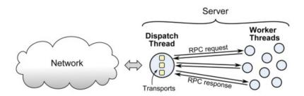
Figure 7.1 – The dispatching-workers threading architecture [taken from [86]].
