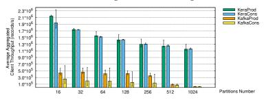
**Figure 8.8** – Evaluating the ingestion component when increasing the number of partitions/streamlets. Parameters: 4 brokers; 16 producers and 16 consumers; *request.size* = 1 MB; *chunk.size* equals *request.size* divided by the number of partitions per broker.
