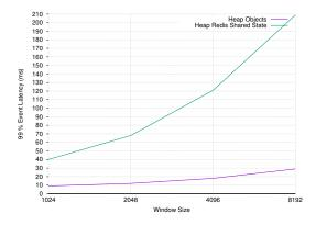
**Figure 4.4** – Event processing latency (99% percentile) for fixed event rate when varying the window size (heap versus shared). Rate of new events is 60. Heap size is 1 GB. Parallelism is one: all events correspond to the same window.
