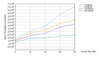
**Figure 8.11** – Baseline: average throughput per client with replication disabled. The configuration with 16 clients (8 producers running in parallel with 8 consumers) corresponds to maximum broker requests parallelism. Increasing the number of clients results in increased competition between producers thus reduced ingestion and processing throughput per client.
