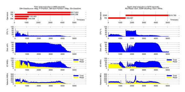
**Figure 3.15** – Tera Sort operators and resource usage of Flink and Spark for 55 nodes and 3.5 TB dataset (similar memory usage).
