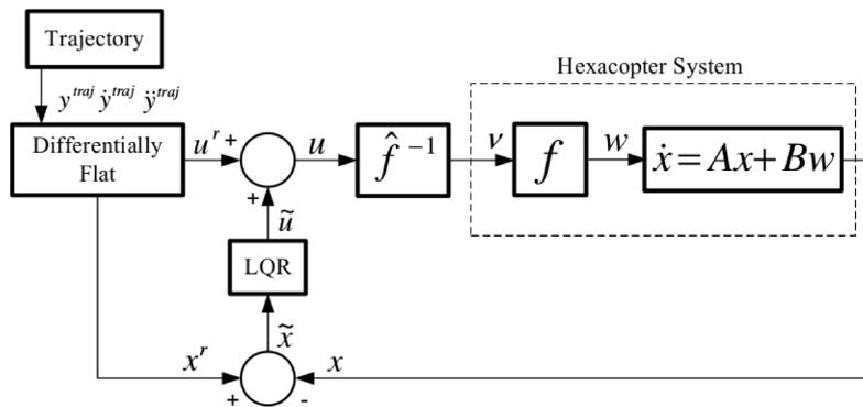
Figure 2.4 – System architecture for LQR control of a hexacopter. A function ( $\hat{f}^{-1}$ ) converts the inputs  $u$  to the actual commands  $v$  fed to the real system (commanded in acceleration with  $w$ ) from [30].
