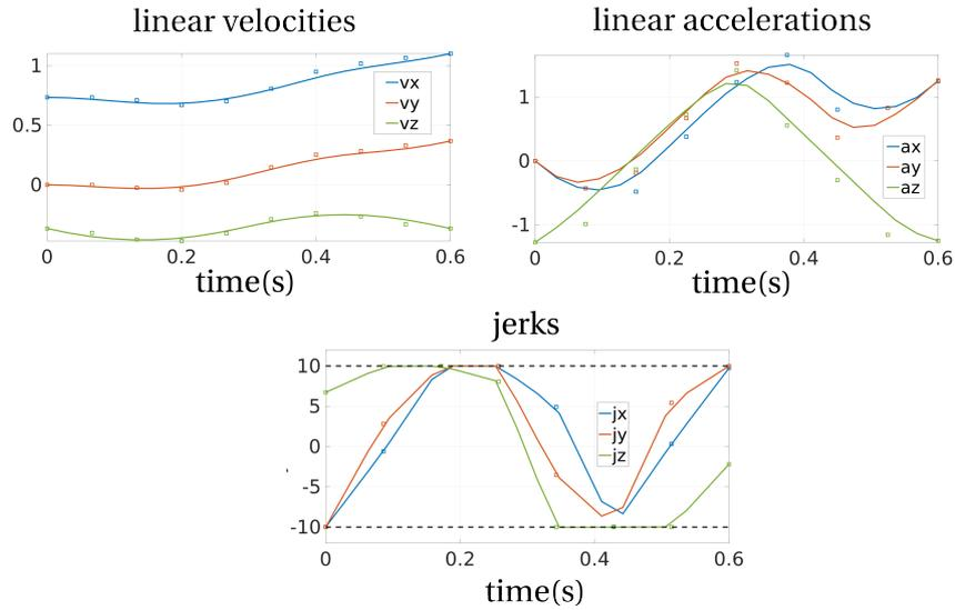
Figure 8.12 – Constrained velocities, accelerations and jerks along the connection trajectory with bounds  $\bar{v} = 2m.s^{-1}$ ,  $\bar{a} = 4m.s^{-2}$  and  $\bar{j} = 10m.s^{-3}$ . The small squares represent the B-spline control points.
