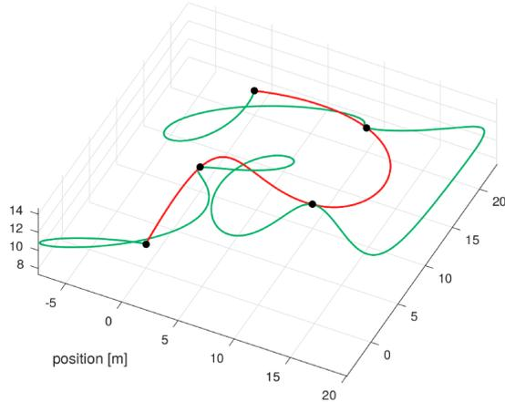
Figure 8.3 – A minimum snap (red) passing through waypoints and a trajectory (green) yielding well-observable states. This trajectory is much longer and much more complex, from [209].
