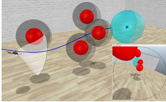
Figure 7.1 – An optimal trajectory for a quadrotor equipped with a camera is generated for reaching a minimum distance with a target (blue sphere) while avoiding collisions with spherical obstacles (inflated dark spheres) and occlusions of the target from the obstacles (red spheres).
