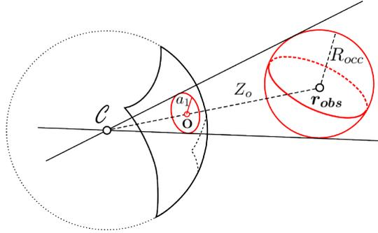
Figure 7.2 – The spherical projection of a sphere in the image of a camera at position  $\mathcal{C}$  is a circle of radius  $a_1$ .
