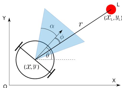
Figure 8.2 – A unicycle equipped with a fixed camera receives position measurements updates whenever a visual landmark (red dot) is close enough and enters the field of view.
