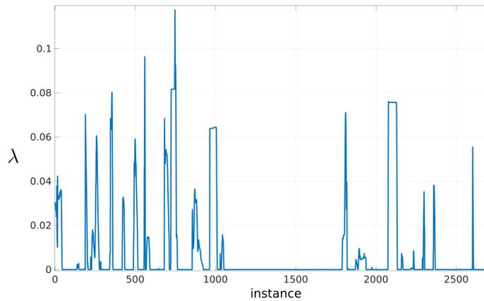
Figure 7.5 – Evolution of  $\lambda$  for the simulation. The peaks reveal the presence of sudden occlusions. The flat section (from around instance 1100 to instance 1700) represents a flight period when the target is far from the obstacles. Therefore,  $\lambda$  is very close to 0. Here  $\lambda$  did not hit the upper limit  $R_{occ} = 0.15m$ .
