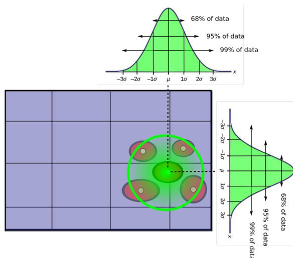
(c) If the green 3-sigma ellipse is fully contained in the field of view, the landmark is guaranteed at 99% to be visible at a given time instant (in theory).
