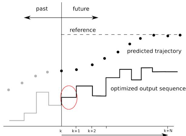
Figure 4.1 – At time  $k$  the future sequence of control variables is computed based on the prediction of the future states. Then the first value of the optimal control sequence is applied to the system (circled in red). At time  $k + 1$  the optimization is repeated with the same prediction horizon.
