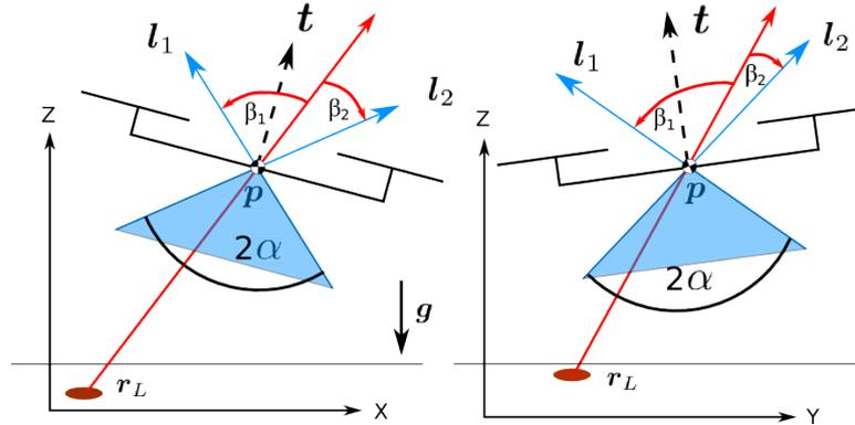
Figure 8.6 – The quadrotor in the vertical planes X-Z and Y-Z with  $\psi = 0$ . For simplicity let us assume that the robot COM  $p$  corresponds to the camera position. Having uncertainties on the state affects the visual perception. To evaluate if a landmark (red blob) is visible under the state uncertainty we check that condition (8.19) is satisfied on both planes.
