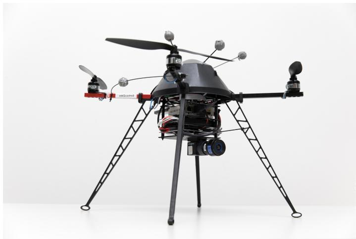
Figure 1.2 – A classic quadrotor platform (from MikroKopter<sup>2</sup>) used for our experiments.
