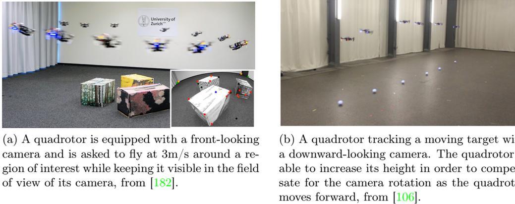
(a) A quadrotor is equipped with a front-looking camera and is asked to fly at 3m/s around a region of interest while keeping it visible in the field of view of its camera, from [182].
