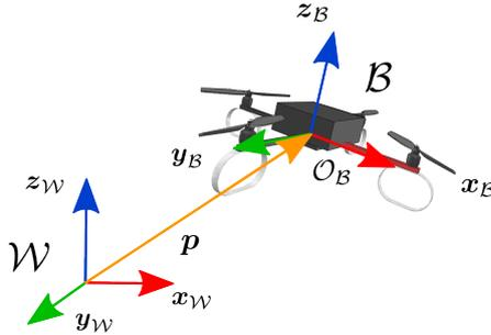
Figure 8.4 – Quadrotor model
