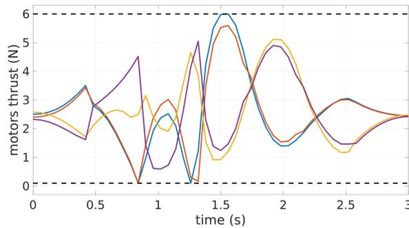
Figure 6.3 – Example of (bounded) motors thrust profiles considering a parametrization of the flat outputs with a 4-th order B-spline basis.
