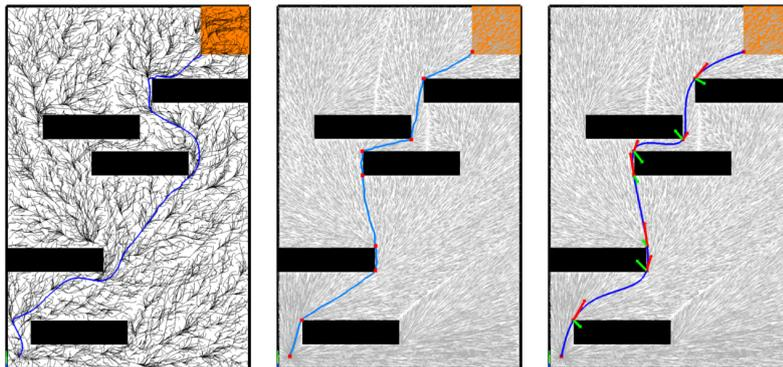
Figure 5.4 – A path is built from a straight-line RRT\* (middle figure) and then refined to obtain a minimum-snap trajectory that is feasible for the real system (right figure). The approach is much faster than a RRT\* with a polynomial steer function (left figure), from [75]).
