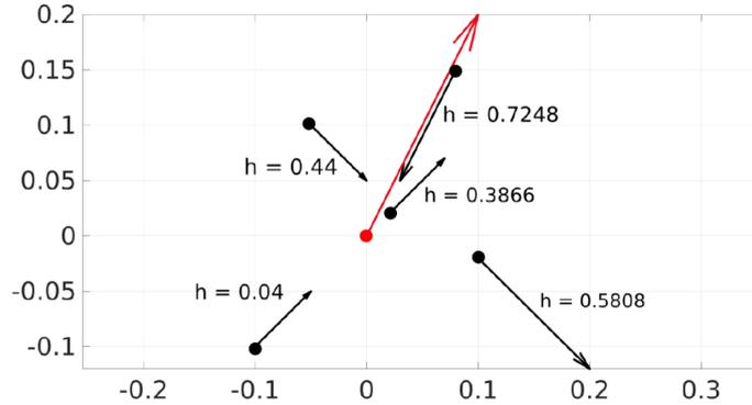
Figure 8.10 – Computation of the heuristic cost  $h(s_1, s_2)$  between multiple vertices  $s_1$  and a goal vertex  $s_2$  at the origin. The arrows represent the vertices linear velocity. As we can see the vertex with the lowest cost is the one whose velocity vector is the most “aligned” with the goal velocity vector. Vertices that are closer to the goal have a higher cost.
