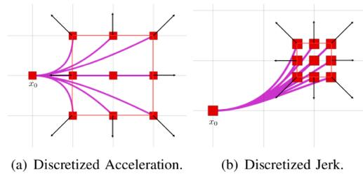
Figure 5.2 – Example of motion primitives from an initial state for an acceleration-controller system (left) and a jerk-controller system (right). The black arrow indicates the corresponding control inputs, from [147].
