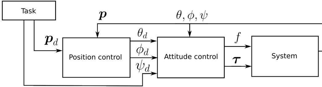
Figure 2.2 – Classic two loop controller. A task provides the desired position  $\mathbf{p}_d$  and yaw angle  $\psi_d$ . The position controller generates the required pitch and roll angles to the attitude controller which applies the computed input thrust and torques to the system.
