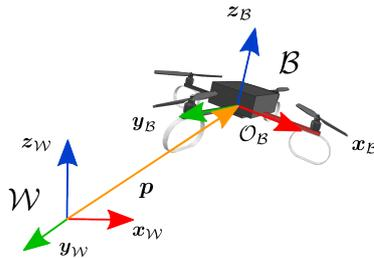
Figure 2.1 – Quadrotor model
