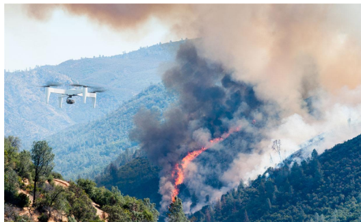
(c) Prelaunch units of the new quadrotor US-1 developed by Impossible Aerospace have been sold to firefighters, police departments, and search and rescue teams across the United States. The system could carry thermal cameras or multispectral sensors for search-and-rescue applications.
