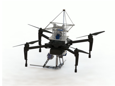
(b) The SpiderMAV uses an air-compressed module to shoot hooks attached with wires to stabilize itself, from [20].
