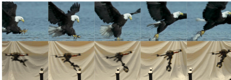
Figure 5.8 – Aggressive catching manoeuvres at 3m/s in the sagittal plane using a monocular camera. The catching strategy is inspired from the natural behaviour of the bald eagle snatching its prey, from [160].
