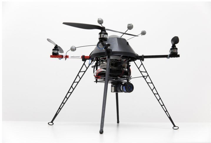
Figure 1.2 – A classic quadrotor platform (from MikroKopter 2 ) used for our experiments.
