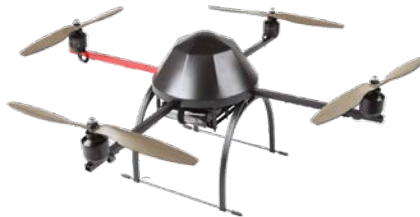
Figure 1.2 – A classic quadrotor platform (from MikroKopter 2 ) used for our experiments.
