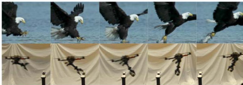
Figure 5.8 – Aggressive catching manoeuvres at 3m/s in the sagittal plane using a monocular camera. The catching strategy is inspired from the natural behaviour of the bald eagle snatching its prey, from [158].
