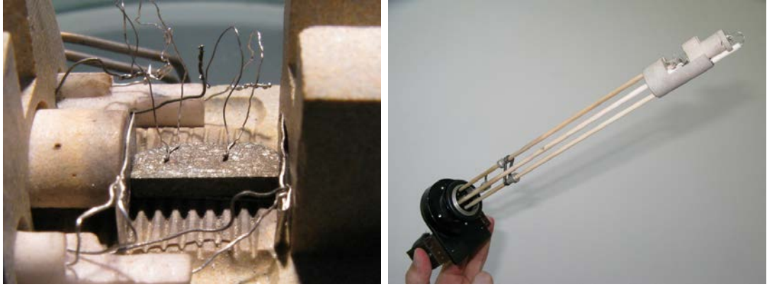
Figure 3.6: High temperature experimental setup for measuring \rho and S . The whole assembly is placed in a furnace.
