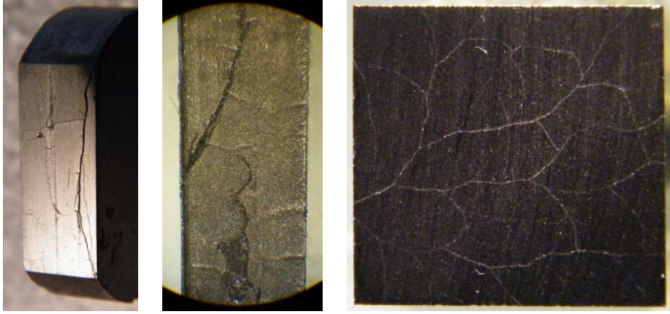
Figure 4.75: Photos showing the defects in sintered samples of doped \text{CaMnO}_3 .
