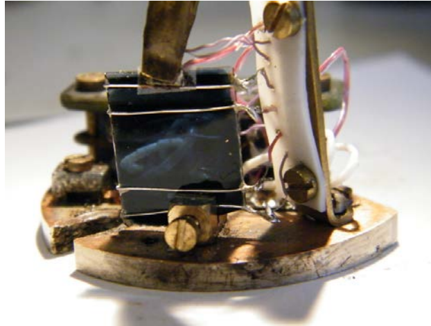
Figure 4.87: Photo of a sample holder modified for measuring thin films on a substrate. Here, a PEDOT:PSS sample is mounted. The heater at the top of the sample is temporarily being held in place by a peg, while the glue attaching the heater is drying.
