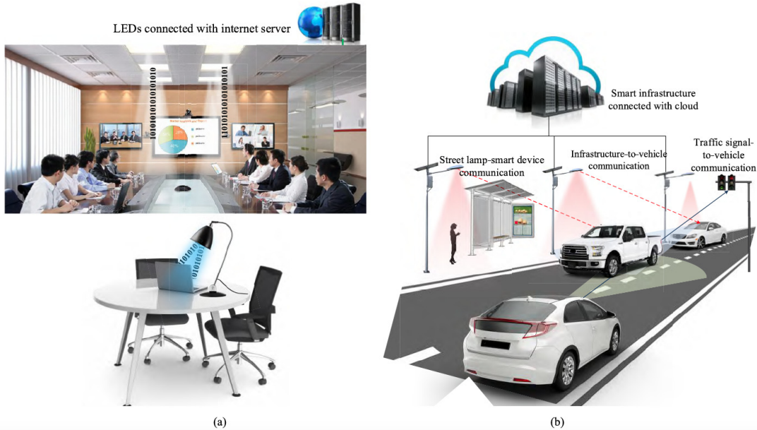
FIGURE 1.7: Application scenarios for VLC/LiFi; (a) indoor applications and (b) outdoor applications [15].
