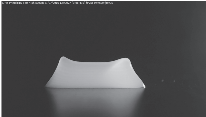
Figure 3.9.: Image of 45wt% boehmite gel printed after aging for more than 4h. Despite a supposedly sufficient yield stress of 200 Pa, as calculated in Eq.3.4, the gel is clearly slumping. The shape of this object clearly confirms that yield stress is not a sufficient criterion to assess the printability of a DIW ink.
