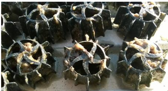
Figure 27 Biofilm growth on Biofill Type C ®
