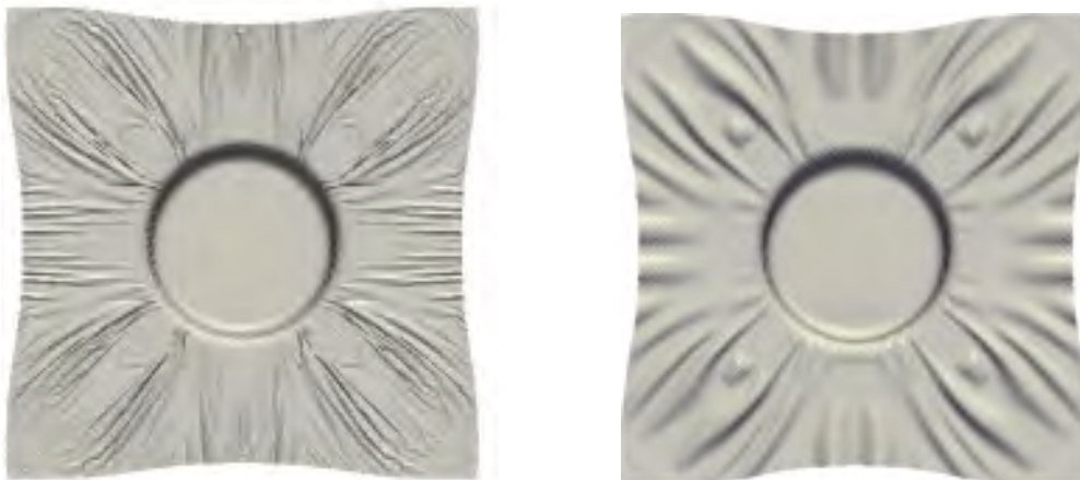
(a) Simulation without bending stiffness (b) Bending stiffness is considered in the simulation
