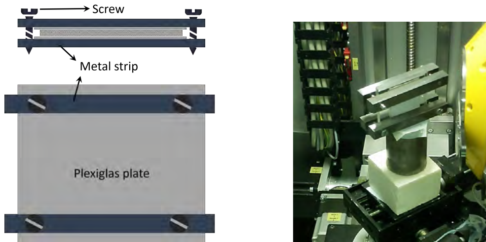
FIGURE 2.10 – The experimental setup for the tomography of compacted tapes stacks
