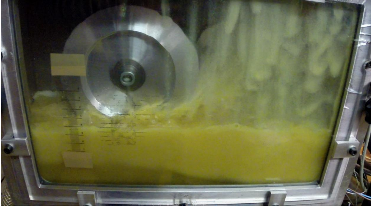
Figure 38: oil behavior in LabECAM test rig (oil A, 3000 RPM, 70°C)
