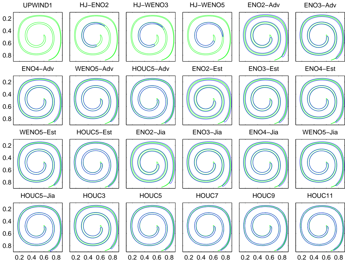
Figure 1.22: Volume constraint: shearing vortex interface at time t = T/2 = 3 with the different advection schemes on a 100^2 grid with CFL = 0.5 . the HJ-ENO2 scheme for the reinitialization. \Delta\tau = \Delta x/2 , \tau_{\max} = 2\Delta x and N_{\text{reinit}} = 1 . Green: Exact interface ; Blue: Volume constraint.
