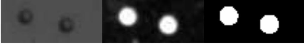
*Figure 4.15:* Pictures showing different stages of image processing technique where the artificial increase in diameter is observed.
