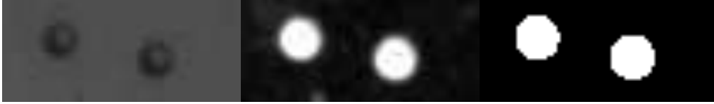
Figure 4.15: Pictures showing different stages of image processing technique where the artificial increase in diameter is observed.
