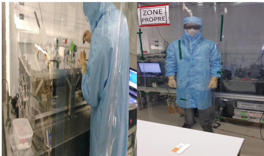
Figure 4.28 During experimental work, one must wear a hat, gloves and a clean body suit in order to keep clean.
