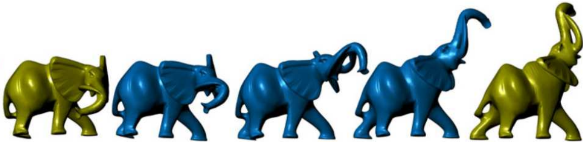
Fig. 3.2 The ARAP interpolation method (ARAPi) applied on an elephant mesh (captured from [147]). The initial and final meshes in yellow are given as input. ARAPi allows to interpolate from the initial mesh to the final one, while maintaining the structure as-rigid-as-possible, resulting in the intermediate poses in blue.
