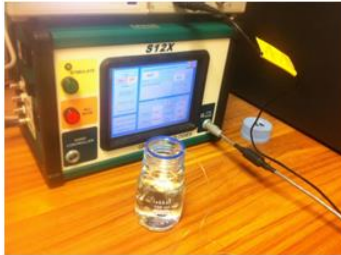
Fig. 4-19. Grass Technologies S12X Cortical stimulator system (Natus Neurology Inc.,USA). Constant-current biphasic stimulator.
