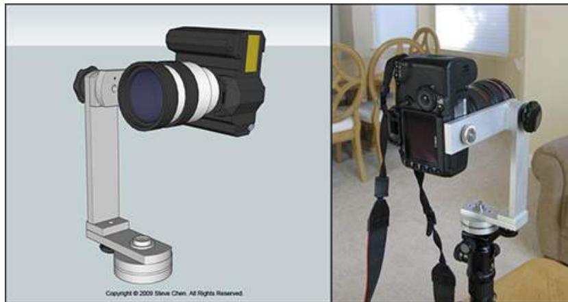
Figure 2.3: Camera gimbal for a parallax-free panorama
