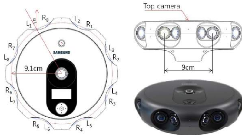
Figure 3.16: Samsung Round 360 VR camera specifications and measurements (Figure taken from [Limonov et al., 2018]).
