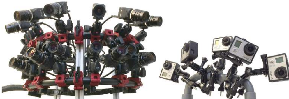
Figure 3.2: An unstructured camera setup used by Perazzi et al. [Perazzi et al., 2015]
