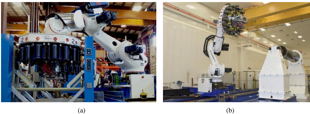
Figure 13 (a) Robot-based AFP system with modular head developed by Electroimpact, ©Electroimpact (b) Robot-based AFP system in the Composites Technology Center of NASA, ©NASA
