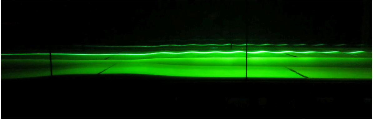
FIG. S3. Picture of the LASER line showing the stationary undulation over the obstacle. The distance between both vertical black lines is 1 m.
