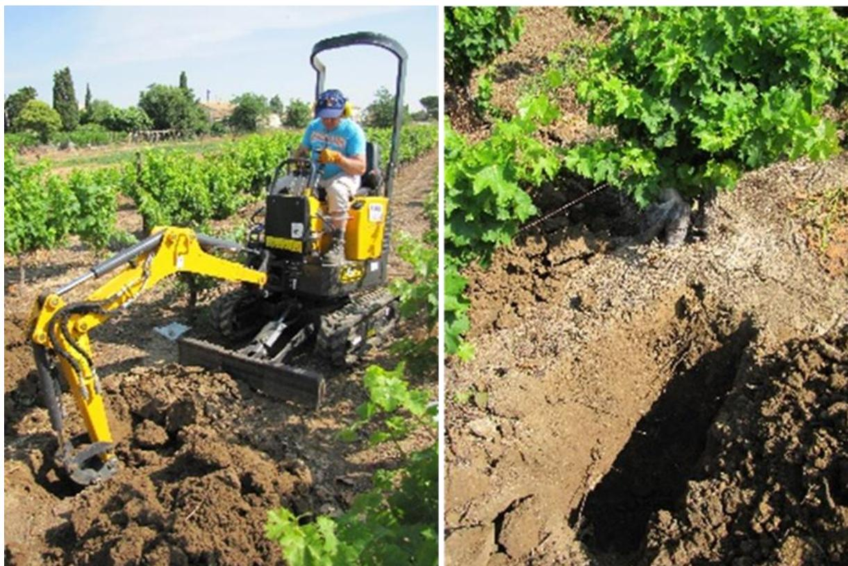
**Figure 3.16.** Soil sampling in the field in trenches, approx. 60-cm deep, 120-cm long and 40-cm wide, dug by a narrow excavator in June 2015. Sampling was performed in the middle part of each replicate (between plants 3 and 4 out of the 6 plants). In each trench, 2 sub-samples of 2 kg of soil were taken by hand.
