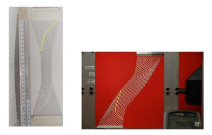
Figure 11: Single fibers undergo large deformations in standard extension test (left) as well as in a shear test (right). Two fibers have been hoghlighted in yellow to show the deformation. Notice in particular that the overall deformation in the left figure is quite moderate and still the highlighted fiber clearly undergoes geometrically nonlinear deformations (the test in the right picture has been described in [4]).
