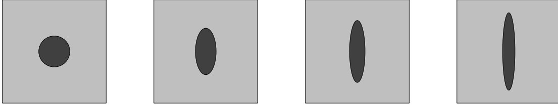
Figure 4.19 – Meshed views of the microstructures under consideration, with b/a \in \{1, 2.25, 4, 6.25\} from left to right.
