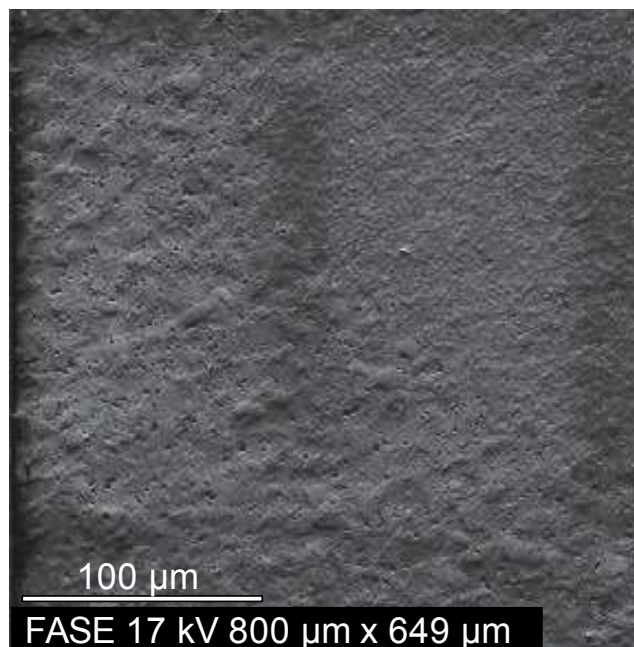
Fig. II-10 Example of the effects of electrostatic chargeup during EBSD. Previously analyzed areas appear brighter. Higher levels of charging will lead to skipped rows, warping and other artifacts.
