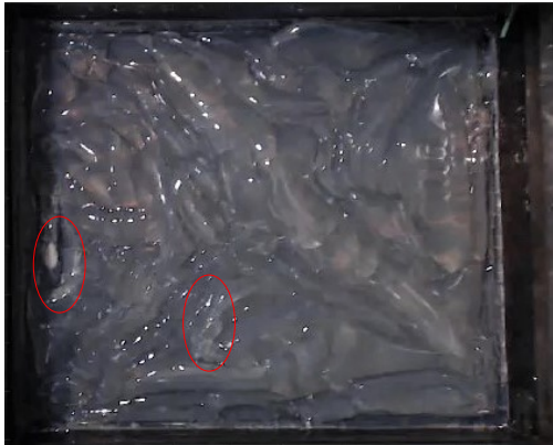
(c) Zone 2: the glass transition starts to take place and white, solid material appears (red circles).
