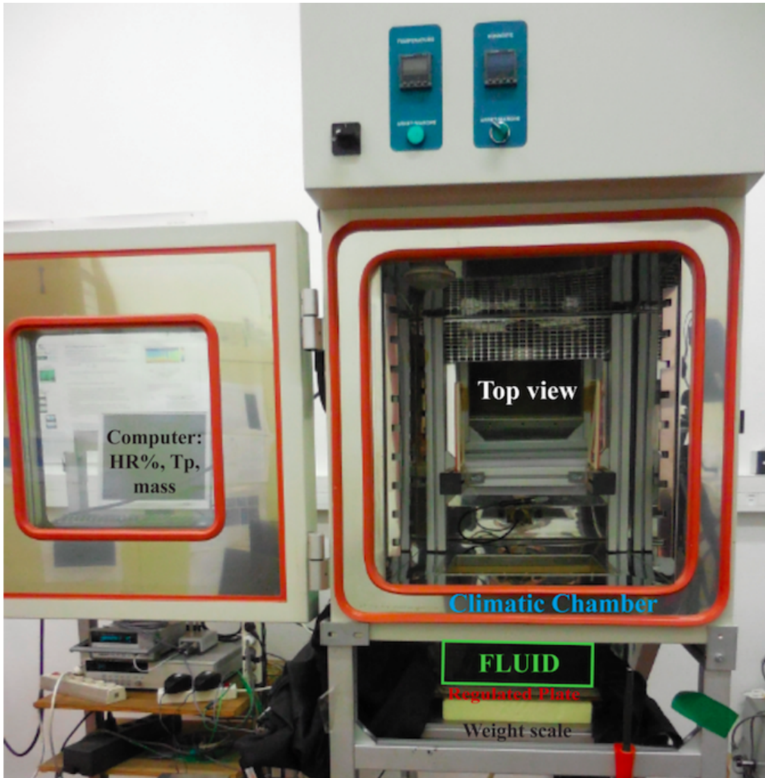
Figure 5.3. Experimental setup of a drying convection experiment. The colloid layer into the tank (green) is dried from above by an air stream whose temperature ( T ) and humidity (Rh) are controlled by a climatic chamber. For our experiment is T = 25^{\circ}\text{C} and \text{Rh} = 30\% . The tank is placed on a metal plate that can be heated if needed. Further below there is a weight scale that records the mass lost during the experiment because of the evaporation of water.
