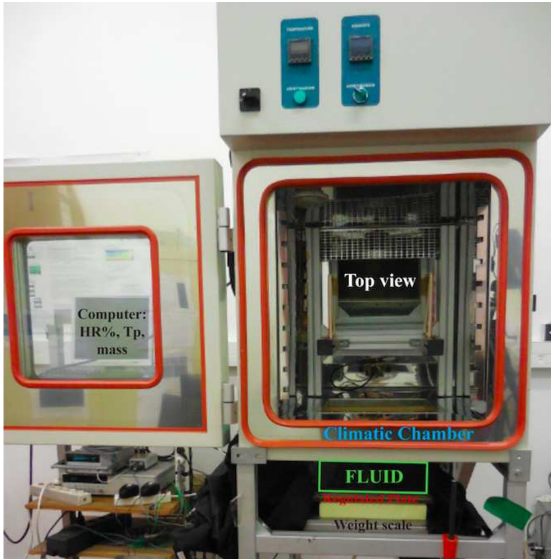
Figure 5.3. Experimental setup of a drying convection experiment. The colloid layer into the tank (green) is dried from above by an air stream whose temperature ( T ) and humidity ( R_h ) are controlled by a climatic chamber. For our experiment is T = 25^\circ\text{C} and R_h = 30\% . The tank is placed on a metal plate that can be heated if needed. Further below there is a weight scale that records the mass lost during the experiment because of the evaporation of water.
