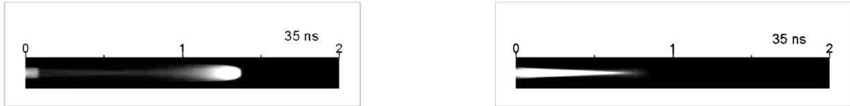
Figure I.5: Image plots of normalized N_2(C-B) radiation intensity for positive (on the left) and negative (on the right) voltage polarity from Naidis [2011a].
