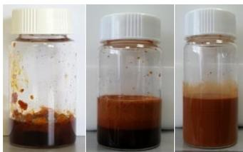
Figure 3.6. Nanodispersions obtained after HPH process with FF-cit (left), FF-CMD (middle) and FF-PAA or FF-PAAMA (right).
