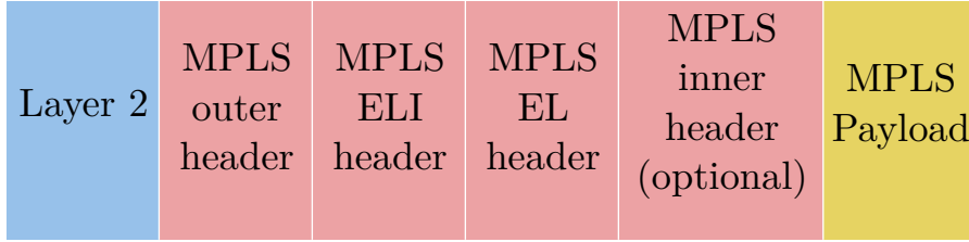
Figure 3.4 – MPLS datagram containing an Entropy Label (EL)
