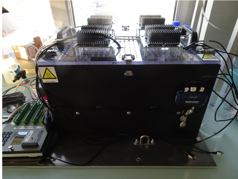
Figure 4.32: New lighting system installed on the enclosure - Side View
