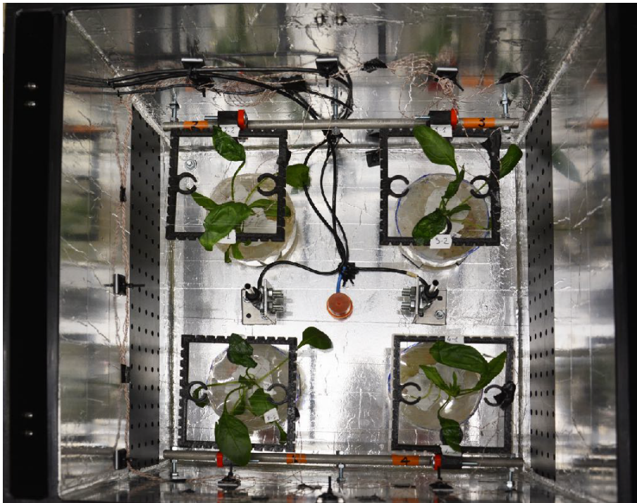
Figure 4.4: Inside the enclosure: Spinach plants under 3D printed frames equipped with hygrometer holders and nylon thread to hold the leaves horizontally. On both sides, the perforated plates are shown.
