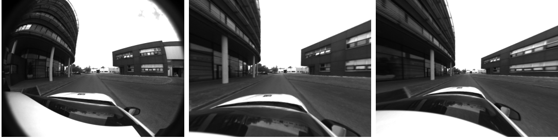
Figure 4.2: From left to right: Original fisheye image and two undistorted versions. In the second image the scale of the neighborhood of the projection center is preserved, in the third one it is compressed in order to capture a wider field of view.
