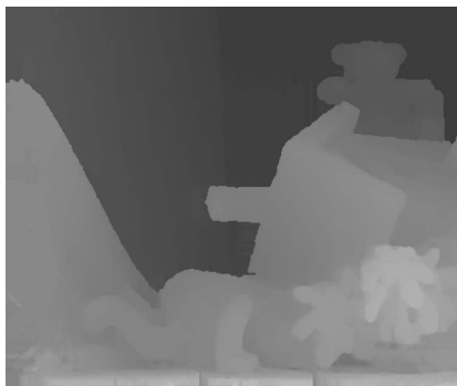
Figure 4.4: Semi-Global Matching (image from Hirschmuller (2008)). The result is much more regular than the ones presented in Fig. 4.3.
